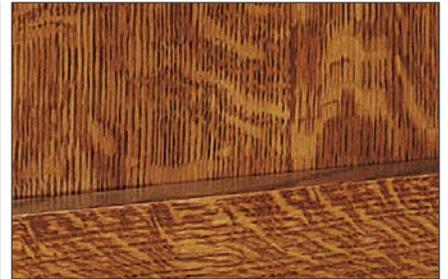
Quarter Sawn is created by using a different sawing technique to expose the different grains in the wood bringing out the flakes that remind us of family heirlooms.
