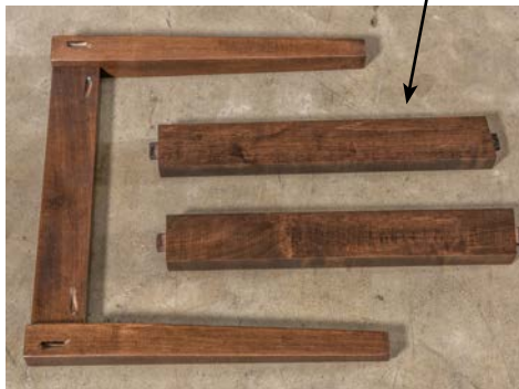
leg assembly glued & pocket-screwed
