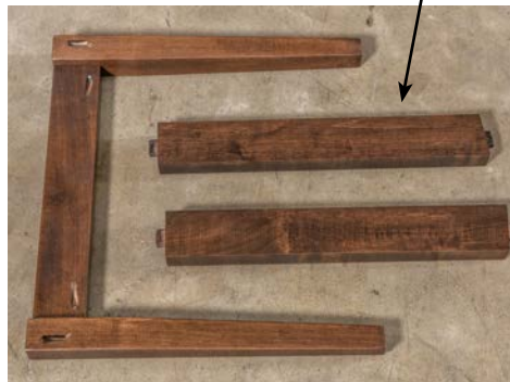
leg assembly glued & pocket-screwed
