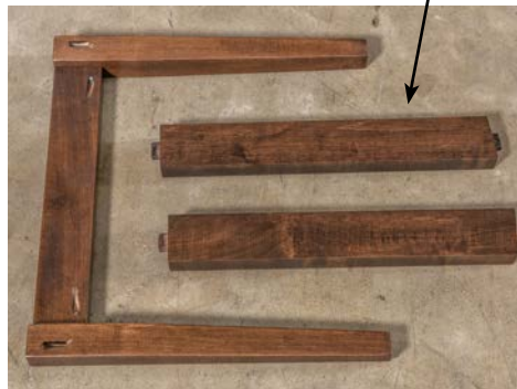
leg assembly glued & pocket-screwed
